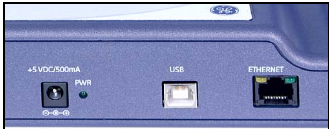
Figure 1-5: Base Station Connections
